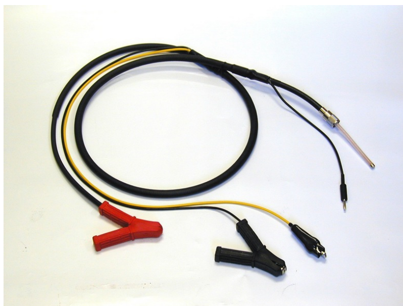
Figure 4: High voltage triaxial test leads assy
